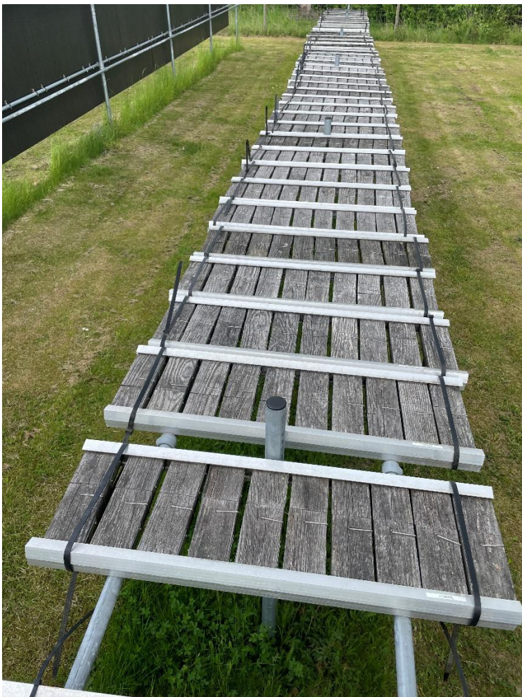
Figure 2: Exposure of the CEN/TS 12037 samples (lap-joints) at the DTI test site in Taastrup, Denmark (left) and NOWA samples in detail, lap-joint clapped open (Photos from May 2026)
