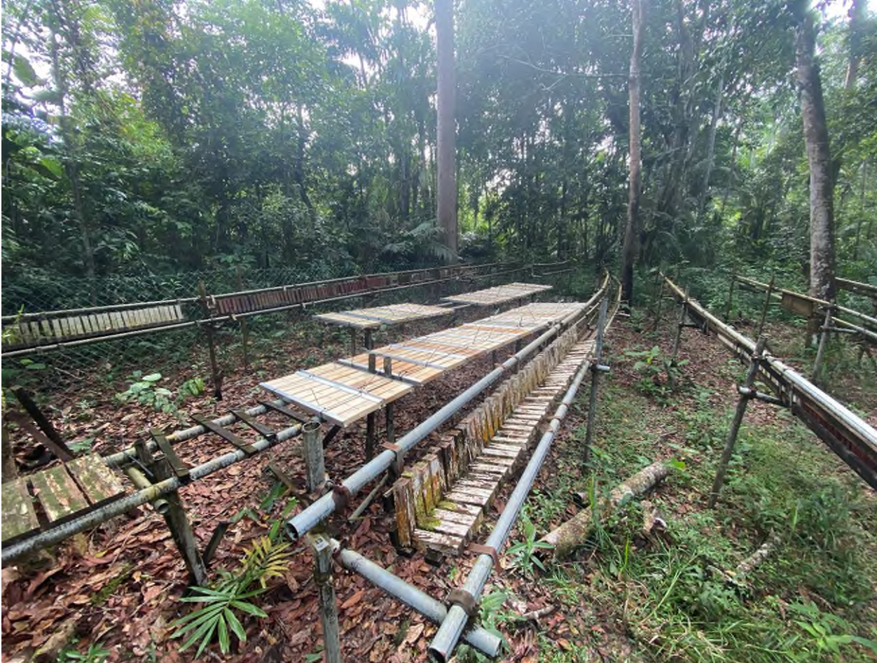
Figure 2: Exposure of the CEN/TS 12037 samples (lap-joints) at the test site in Malaysia
