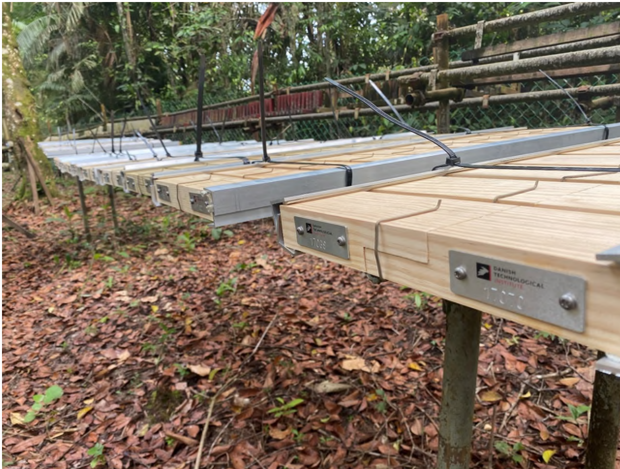
Figure 1: Exposure of the CEN/TS 12037 samples (lap-joints) at the UNIMAS test site in Malaysia
