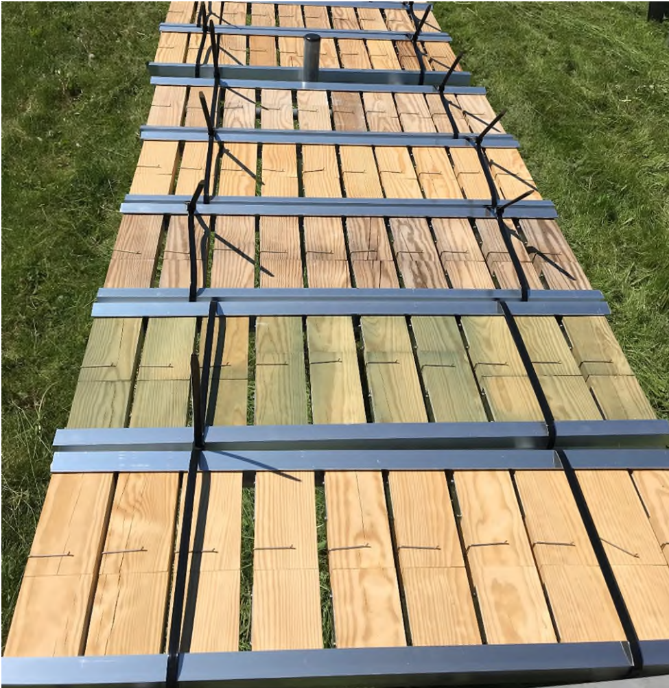
Figure 2: Exposure of the CEN/TS 12037 samples (lap-joints) at the DTI test site in Taastrup, Denmark
